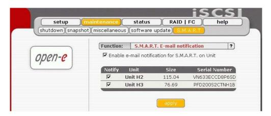
In order to enable S.M.A.R.T. e-mail notification, you have to first enable E-mail notification function in setup -> administrator menu, then enable S.M.A.R.T. in Console tools at special options (press F1 on console to find out keyboard shortcuts).
